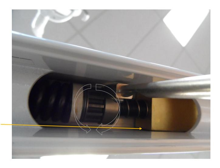
Pull the rod in this direction to allow for rotation of the rod assembly in order to tighten or loosen the spring tension.
