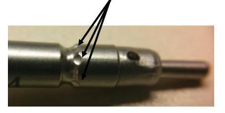
When inserted into the DCI press ring adapter the ball bearings lock into the notches keeping it from rotating freely.
