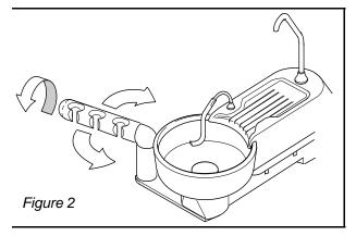
mounting bracket attached to the cuspidor housing.
