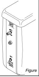
The post mounted utility is equipped with a self-contained water supply. The system can also run on city water. Desired supply is selected with a toggle, labeled "water supply", located on the front panel of the post mounted utility, below the quickdisconnect water outlet.
