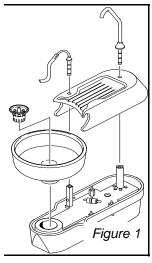
**Cup Filler** The cup filler on the cuspidor is operated by a momentary toggle. As you face the cuspidor bowl, there are two momentary toggles on the lower right side of the cuspidor housing. The toggle for the cup filler is toward the rear. Pull and hold the toggle toward you to turn the water on. Release the toggle to turn the water off.
