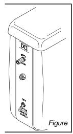
Desired supply is selected with a toggle, labeled "water supply", located on the front panel of the post mounted utility, below the quickdisconnect water outlet.
