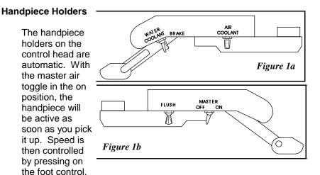
The position of the handpiece holders is adjustable. See the section below on adjustments.
