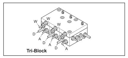
A = Air Coolant, W = Water Coolant, D = Drive Air
