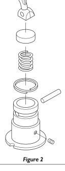
the disc is centered inside the end of the spring. The smooth side of the disc should face up; the toggle rides on this surface.
