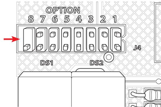
**NOTE:** After setting Base Up and Down, place the jumper on a single pin to prevent loss of the jumper.
