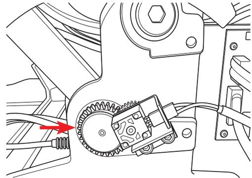
2. Loosen the set screw in the large gear.
