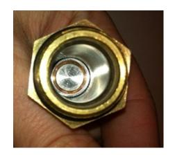
Step 6. Reassemble the purge valve and test for leaking. If it still leaks install a 2166 solenoid repair kit.
